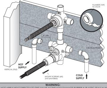
DO NOT APPLY HEAT DIRECTLY TO THE VALVE AS THIS MAY DAMAGE RUBBER & PLASTIC SEALS & WILL AVOID WARRANTY. TURN ON WATER SUPPLIES TO VALVE & CHECK FOR LEAKS
