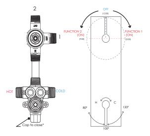
1-132 THERMOSTATIC VALVE W/ 2 WAY DIVERTER
