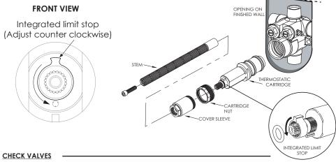
Shut off water supply at main or upstream from valve body. Remove check valve nut with a 5/8" (16mm) socket wrench from the body.
