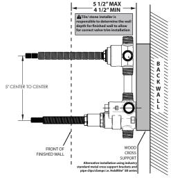
Pre-assemble fittings before attaching to cross support. Attach the "COLD" Inlet to Cold Supply & "HOT" Inlet to Hot Supply using copper supply lines.
